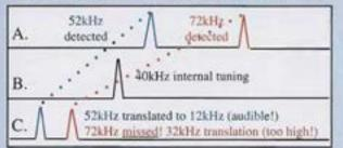
The <u>difference</u> between these two signals is what gets heard in the headset (C). One problem (as seen here) is that if the *incoming* sound is too far from the *internally generated* frequency the <u>difference</u> is too large (high in frequency) to ever be heard by the user. "Fixed band" systems do not widen the frequency detection range of the instrument, only lock in on one *internally* generated one.
