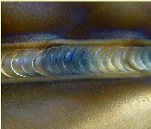
The ferrite level is important to assure minimum exposure to solidification cracking when depositing austenitic stainless steel weld metal. A lower ferrite number is better for corrosion resistance, while balancing higher ferrite content to avoid solidification cracking in the weld
